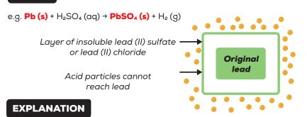
**Insoluble** layer of PbSO₄ formed around lead, preventing further reaction from happening. Reaction terminates prematurely, and the yield decreases.
